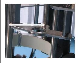
While pressing down the black knob, gently push the upper end of the bottle towards the middle of the rack. When the bottle is in correct position, release the knob and ensure the water sampler is locked in position.
